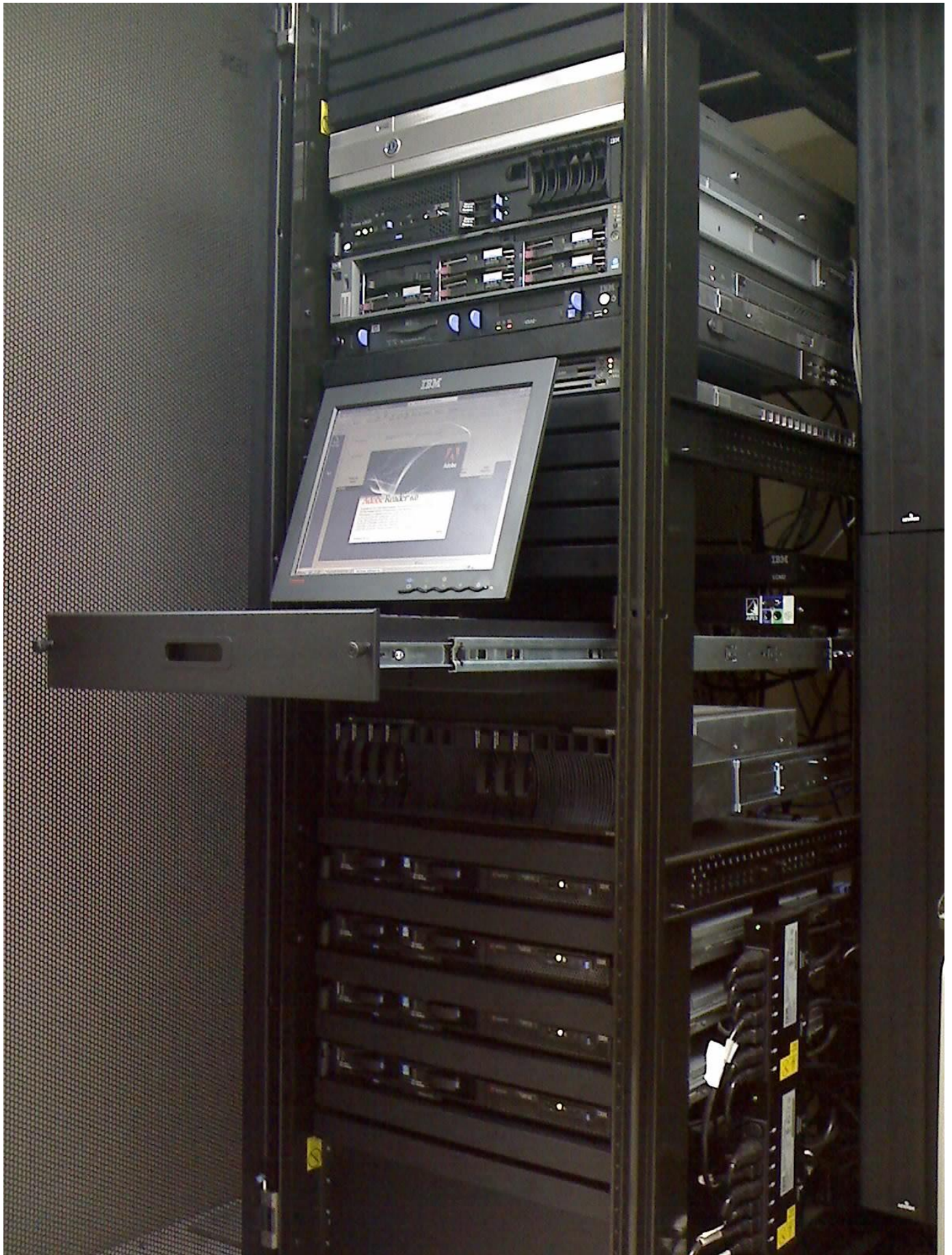
Server Rack with a Console Display
